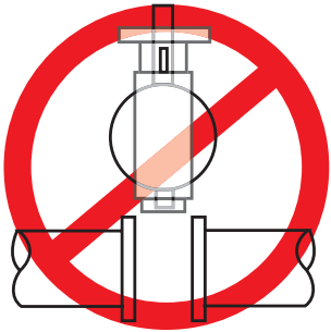
Figure 1 – Insert Resilient Seated Butterfly Valve Between Flanges
